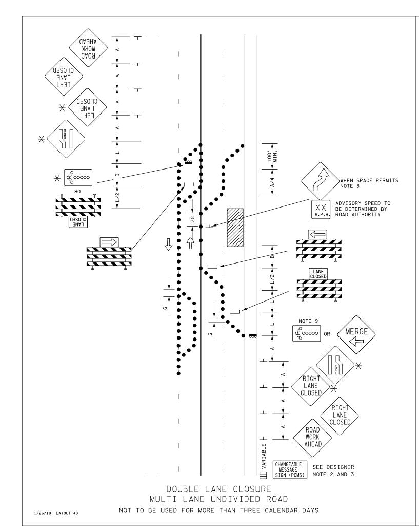
SPACING SPEED DECISION SIGHT DISTANCE ADVANCE CHANNELIZING LENGTH SPACE PRIOR TO WARNING DEVICES (G) (B) SIGNS STARTING (A) (MPH) FEET FEET FEET FEET FEET 550 0 - 30 100 200 200 25 35 - 40 325 700 325 305 45 - 50 600 900 600 425 55 500 750 1200 700 50 60 - 65 1000 1400 800 650 70 - 75 900 1200 1600 820
